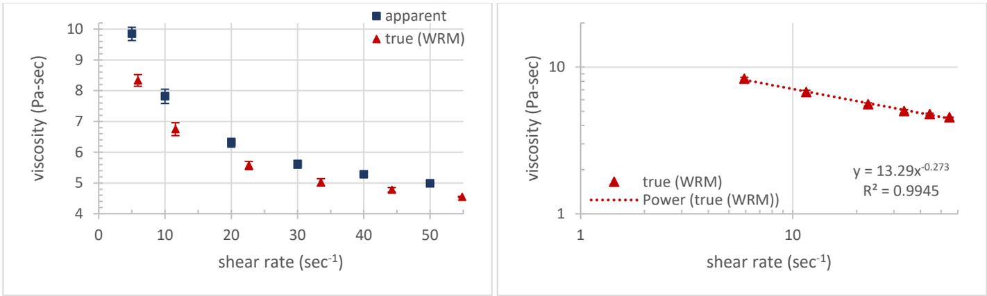
**Figure 1:** Viscosity versus shear rate for WHITE LABS toothpaste. Apparent viscosity is compared to the true obtained after the WRM correction (*left*). The true or corrected viscosity data is shown along with a fit to the power law model (*right*). Error bars represent one standard deviation.
