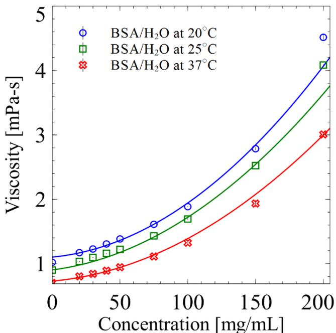
Figure 1. Viscosity as a function of concentration and temperature for solutions of BSA in water. Solid lines correspond to second order polynomial fits (See Table 1 for coefficients).
