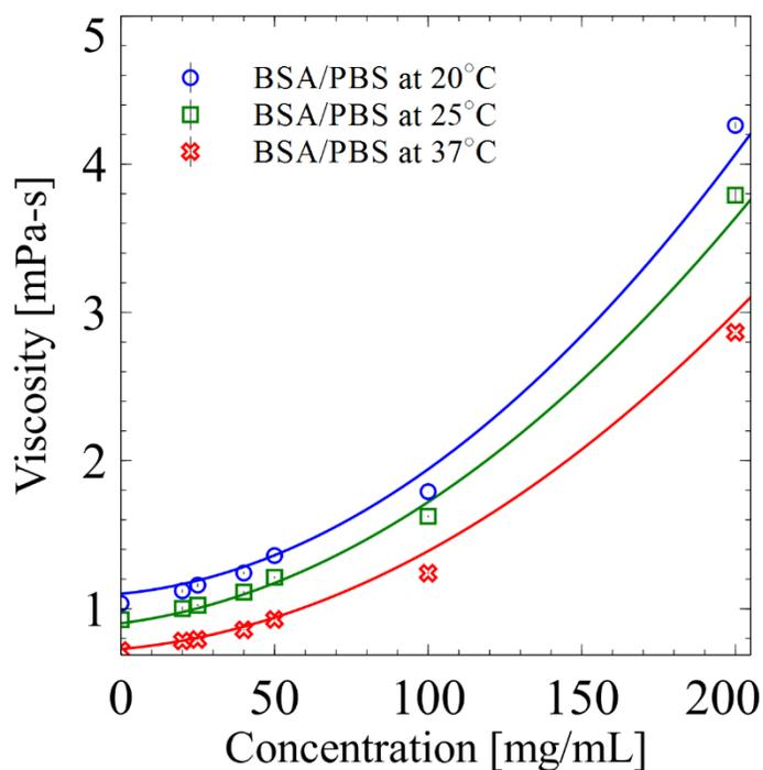
**Figure 2. Viscosity as a function of concentration and temperature for solutions of BSA in PBS. Solid lines correspond to second order polynomial fits (See Table 1 for coefficients).**
