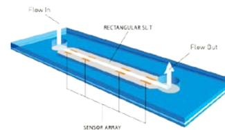
RheoSense's *Viscometer-Rheometer-on-a-Chip* (VROC®) combines microfluidic and MEMS technology to measure viscosity. As the test fluid is pumped through the channel at a controlled shear rate the MEMS pressure sensor array captures the pressure drop, which is proportional to the shear stress at the wall. The viscosity of the test fluid is obtained as the ratio of shear stress to shear rate.
