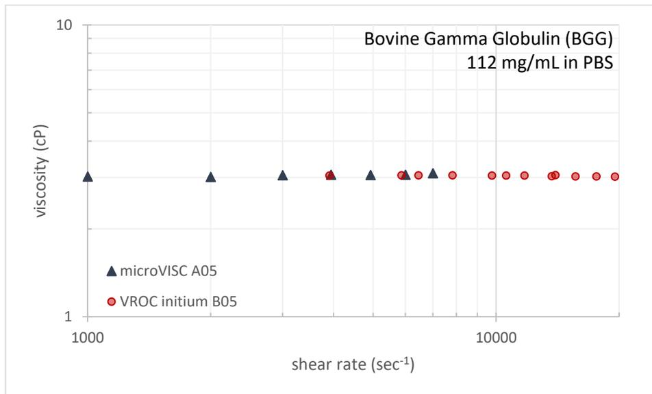
**Figure 1:** Viscosity versus shear rate for 112 mg/mL Bovine Gamma Globulin in PBS at 25°C.
