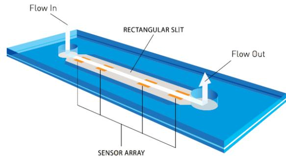
RheoSense's Viscometer-Rheometer-on-a-Chip (VROC®) combines a microfluidic channel with a MEMS pressure sensor array to measure viscosity. As the test fluid flows through the channel the sensor array captures the pressure drop, which is proportional to the shear stress at the wall. The shear rate is calculated from the flow rate and the channel dimensions. The viscosity of the test fluid is obtained as the ratio of shear stress to shear rate.
