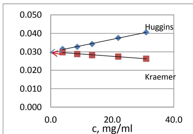
**Figure 2.** Graphical representation on how to obtain intrinsic viscosity using Huggins and Kraemer equations.
